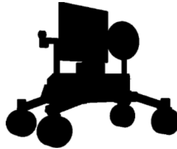
LUVMI: 1.5m x 1m x 1.6m (deployed) Weights about 40 kg
